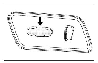
In vehicles with power seats, the controls used to operate them are located on the outboard side of the seat.
